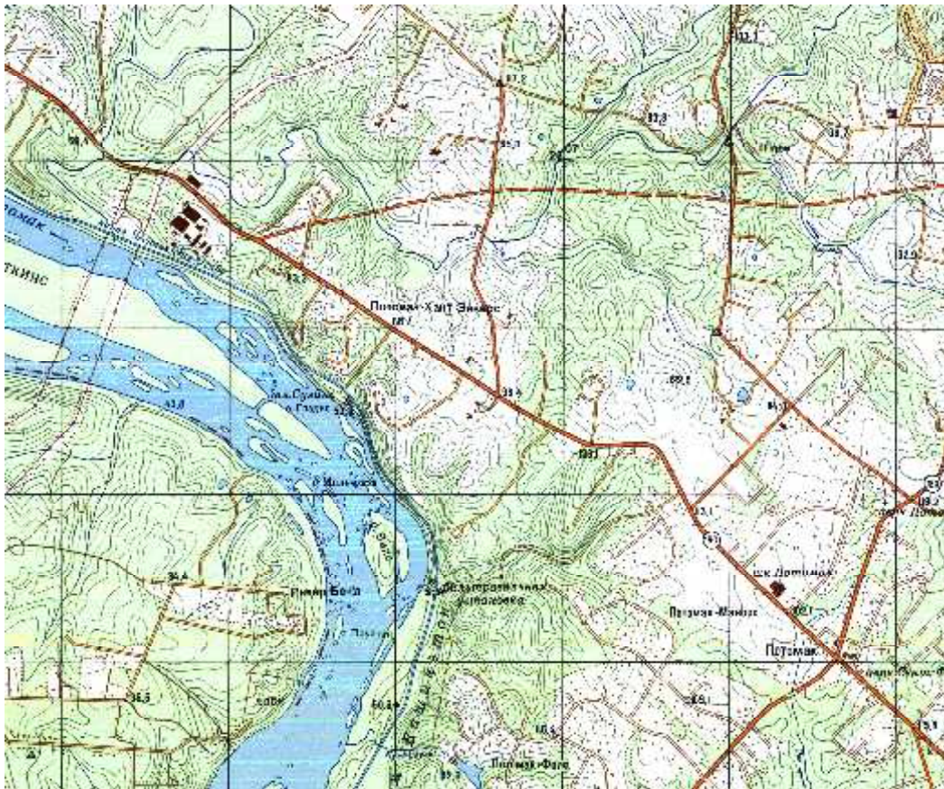
Part of Washington 1:25,000 sheet 1 (compiled 1973, printed 1975) and J-18-A Washington 1:500,000 (compiled 1979, printed 1981) The power transmission line running SW-NE and the road running NW-SE can be seen on both. Spot height of 97.2 on the large scale map is shown as 97 on the small scale sheet. The 'proposed' E-W road has evidently been built and the settlement at the Potomac cross roads has become more substantial.
