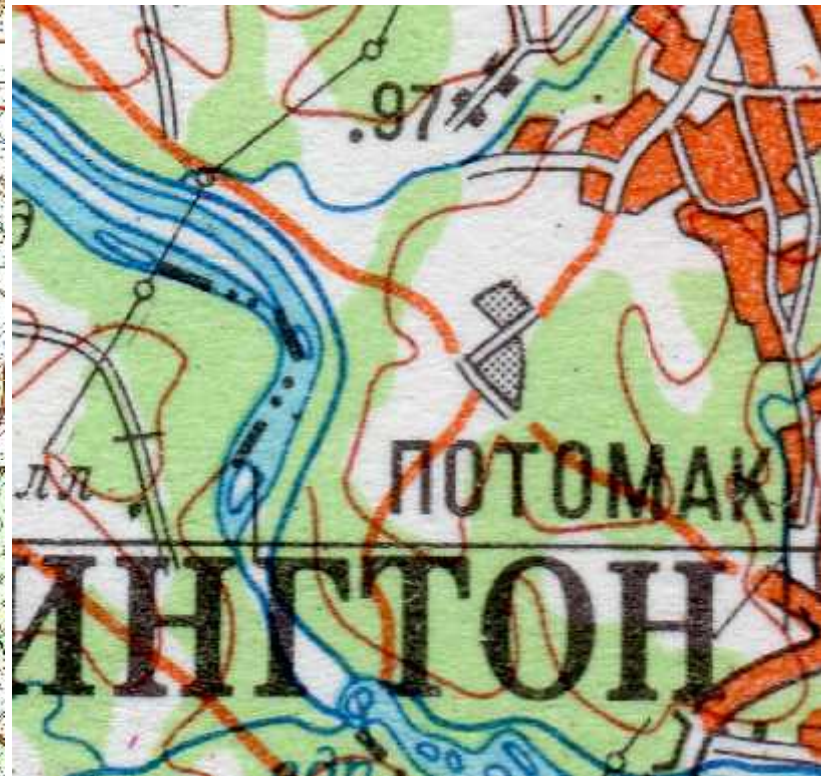
Part of Washington 1:25,000 sheet 1 (compiled 1973, printed 1975) and J-18-A Washington 1:500,000 (compiled 1979, printed 1981) The power transmission line running SW-NE and the road running NW-SE can be seen on both. Spot height of 97.2 on the large scale map is shown as 97 on the small scale sheet. The 'proposed' E-W road has evidently been built and the settlement at the Potomac cross roads has become more substantial.
