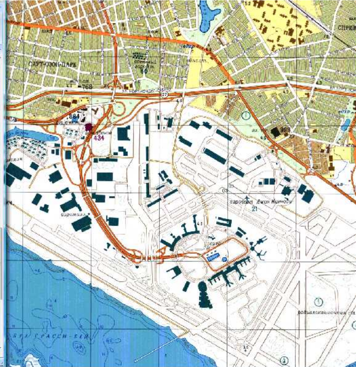
New York - JFK. Note buildings around the terminal loop and northeast of NW-SE runway. Note also SW-NE runway (extending from jetty) shown as complete on 1967 USGS, not yet built on Soviet compiled 1971. Depth 23ft does not convert to 6m, but benchmark 15 is 4.6 and 20 is 6.1 (near top right). Roads and interchange top left are different and urban blocks north and east of airport are differentiated between high rise and low rise.
