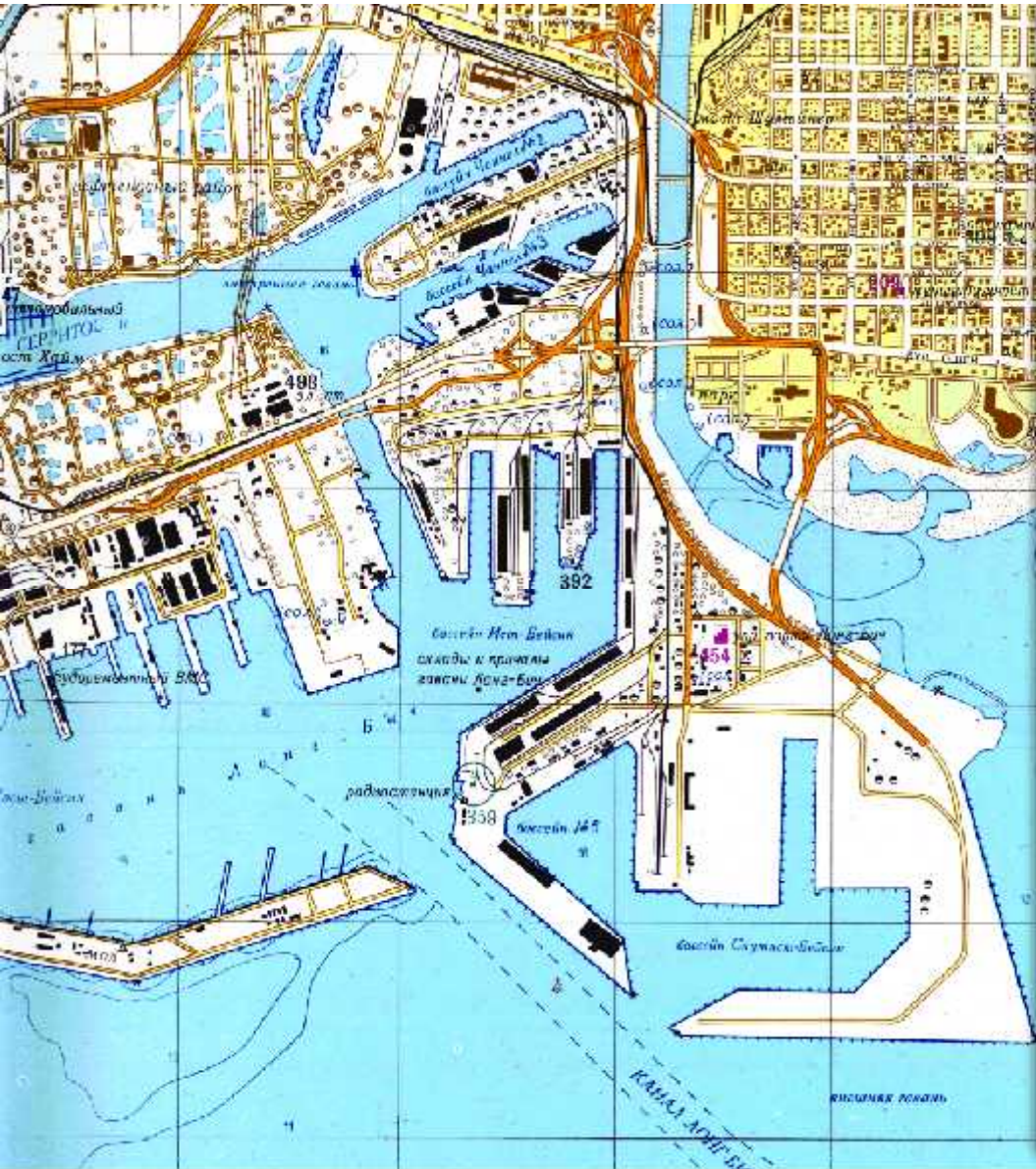
Los Angeles - Long Beach. Note differences such as shape of Southeast Basin and surrounding roads and storage tanks, buildings by Basin Six, bridge, roads and coastline by Rainbow pier, Seaside Blvd roads and bridges. Bathymetric depths do not correspond - 35ft in Basin Six is not 16m, 52ft in Inner harbour is not 17m.
