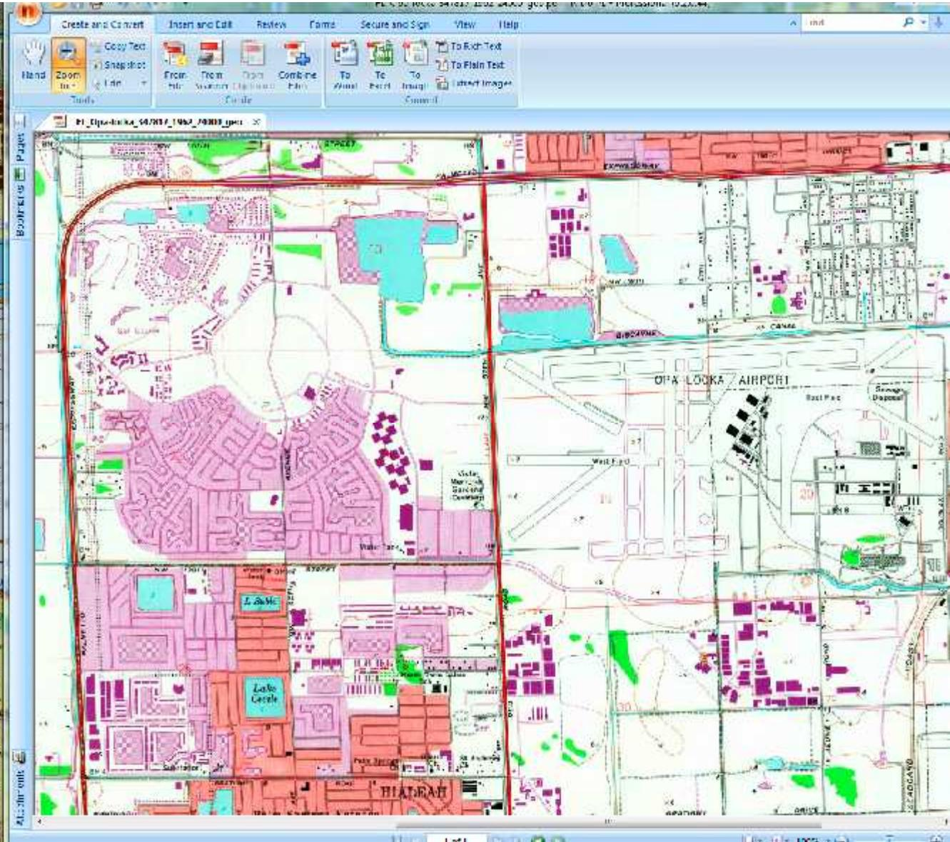
Miami - Opa-Locka. Soviet shows housing developments with street names and ponds not shown on latest USGS. Benchmark 7ft (top right, also by southwest end of runway) converts correctly to 2.1. Soviet also shows elevation of 0.6m at surface level of several small ponds. Object number 100 is listed as plastics factory and 127 as shipbuilding.
